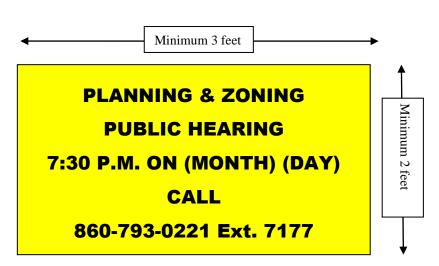
THE SIGN MUST BE MADE OF A DURABLE MATERIAL WITH A BRIGHT YELLOW BACKGROUND AND BLACK BLOCK LETTERING A MINIMIUM 1-3/4" HIGH.
